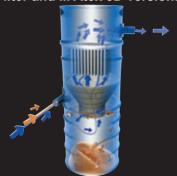
Large-area, coated pocket filter for fine dusts. The unit can be used as "all-round" cleaner for dry or wet suction material.
