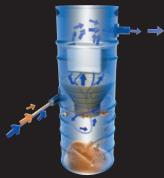
Robust cloth filter made of heavy technical fabric for the extraction of liquids, coarse dust and swarf, e.g. chip removal processing industry.
