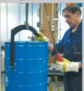
The collection container can be equipped with a transport- and discharge handle. This bar is used to lift the collection container by a crane or forklift truck.
