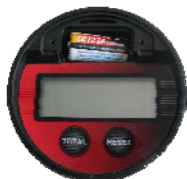
Picture 2: Take out the battery
