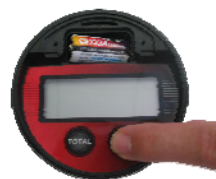
Picture 3: Insert the new battery and press the reset button to check the function of the register
