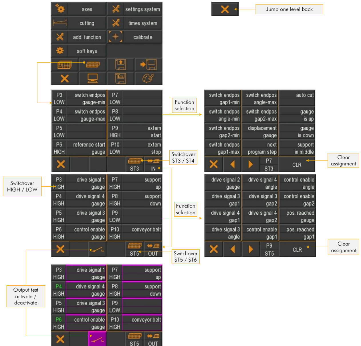
Figure 41: Logic assignment of Input / Output functions
