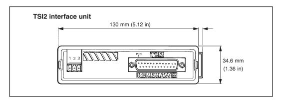
2. A TSI3 interface unit must be used with the Renishaw HPMA.
