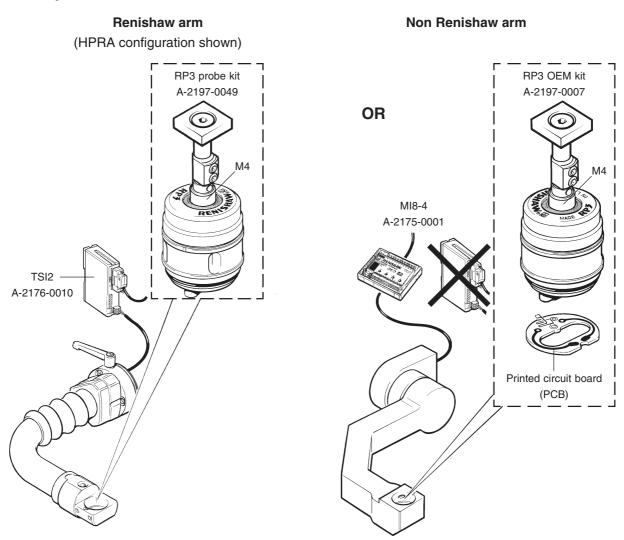
**NOTE:** Check that the RP3 is pressed fully into the probe holder so that the spring pins make electrical contact.
