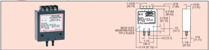
**Series 616 Transmitter** features an exceptional ±0.25% accuracy in several factory calibrated ranges. Choose the one just right for your application. Span and Zero controls included for fine tuning and minor re-calibration in the field.
