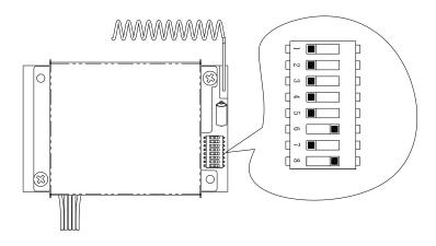
Top slot  $\rightarrow$  "1"; bottom slot  $\rightarrow$  "0" For example : the channel dip-switch set above  $\rightarrow$  00101, channel 05.
