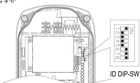
Set the ID codes needed with the dip-switch on the decoder board. For example: the ID codes set above  $\rightarrow$  10000111.
