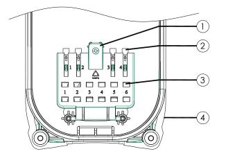
(1)Spare fuse & jumper compartment(2)Spare Jumper slots(3)Spare fuse slots(4)Receiver top casing
