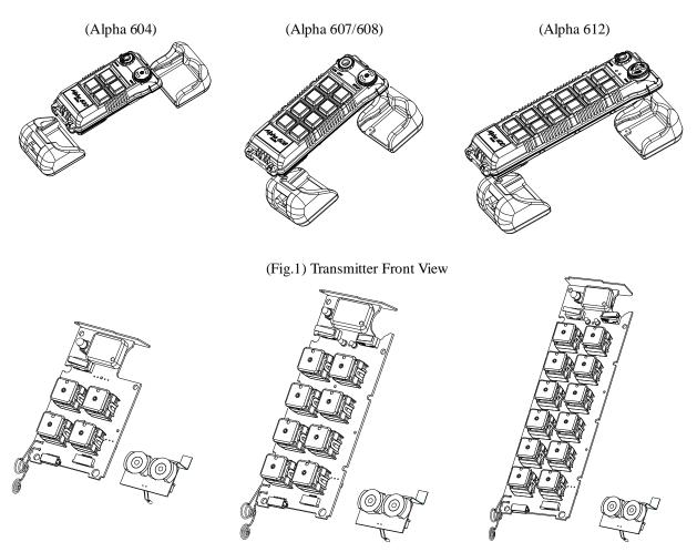
(Fig.2) Transmitter encoder board and induction charging board
