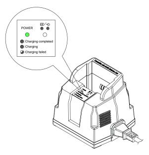
Slide-in transmitter into battery charger (transmitter vinyl protective cover has to be taken off)
