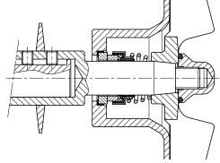
ATTENTION! When installing the new seal, use soapy water when fitting the different parts and gaskets to allow them to slide better; apply to the stationary as well as the rotating parts.
