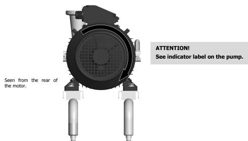
Start and stop the pump motor momentarily. Make sure, looking at the pump from behind, that the motor fan rotates in a clockwise direction.
