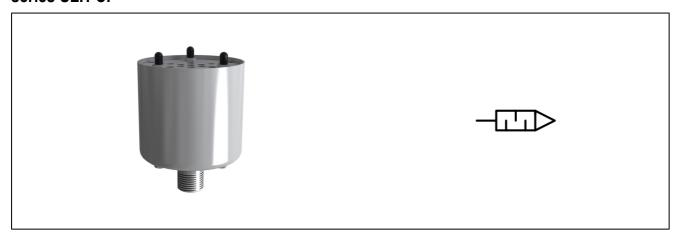
design multi-chamber silencer made of sheet steel with 3 polyester felts thread connections G1/2"...G2" according to ISO228/1 material body steel galvanic zinc plated, perforated sheet zinc plated steel, felts made of polyester function for silencing, high exhaust rate mounting position any medium compressed air, neutral gases -10°C...+90°C medium temperature operating pressure max. 6bar information polyester-felts can be cleaned with cleaning solvent
