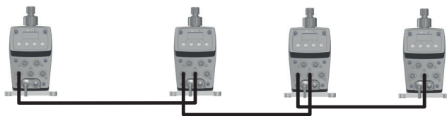
Fig. 29: Synchronization of several dosing pumps by means of stroke feedback and pulse control
