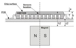
Fig. 23: Magnet placed below AM8192B
