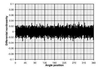
Fig. 15: Typical differential nonlinearity
