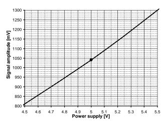
Fig. 28: Signal amplitude Vs Power supply
