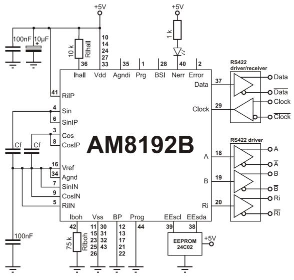
Fig. 34: Typical application scheme
