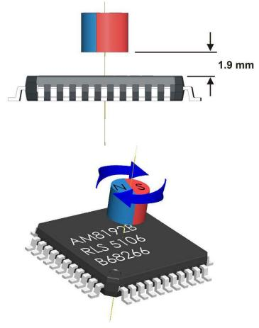
Fig. 1: AM8192B with the magnet
