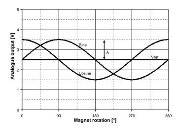
Fig. 5: Timing diagram for analogue output
