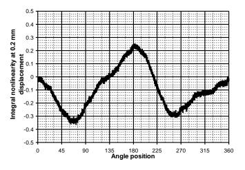
Fig. 17: Typical integral nonlinearity when the chip is displaced for 0.2 mm
