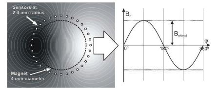
Fig. 19: Distribution of  $B_n$  and its modulation if the magnet is rotated through 360°
