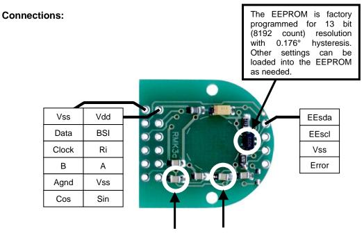
22 nF filtering capacitors – these can be changed as needed.
