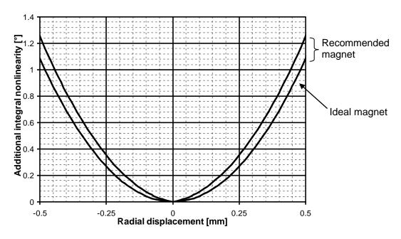
Fig. 21: Additional integral nonlinearity error caused by magnet displacement
