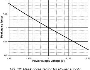
Fig. 12: Peak noise factor Vs Power supply
