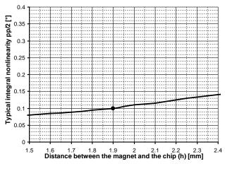
Fig. 31: Accuracy Vs Distance
