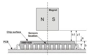
Fig. 22: Magnet placed above the AM8192B
