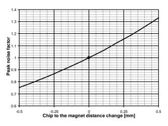
Fig. 14: Peak noise factor Vs Distance change
