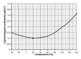
Fig. 33: Accuracy Vs Temperature
