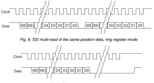
Fig. 9: SSI no ring register mode
