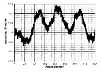
Fig. 16: Typical integral nonlinearity
