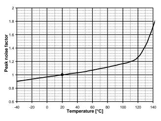
Fig. 13: Peak noise factor Vs Temperature \*
