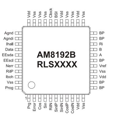
Fig. 2: Pin description for AM8192B
