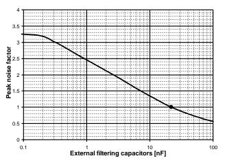
Fig. 11: Peak noise factor Vs Filtering
